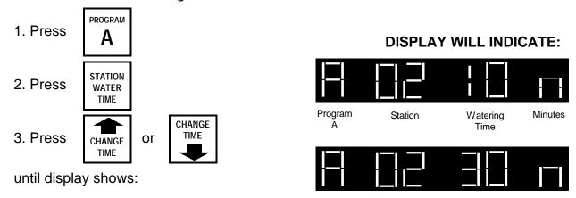
Set watering times for remaining stations by repeating steps 2 and 3. **NOTE:** If you do not want a station to operate, set the time to zero.
