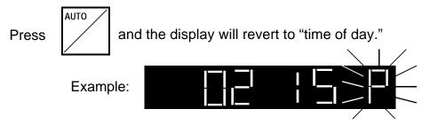
The "A" (A.M.) or "P" (P.M.) character will blink to indicate that the controller is in rain shutdown condition.
